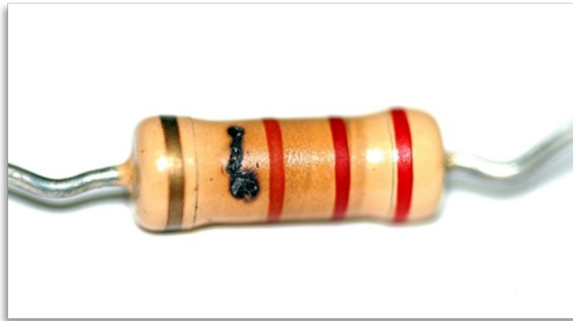
Fig 2.8.1.6: ESD discharge on a resistor
