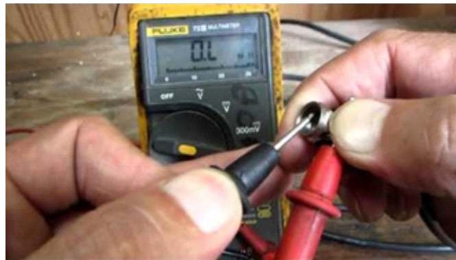
Fig 2.7.2.2: a multimeter being used for checking the coax cable
